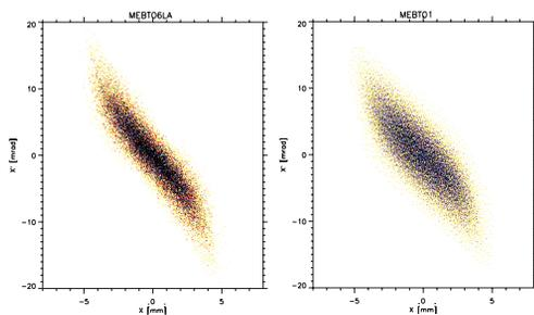
Figure 5: Comparison between original distribution (left) and reconstructed phase space pattern (right) based on MaxEnt.
