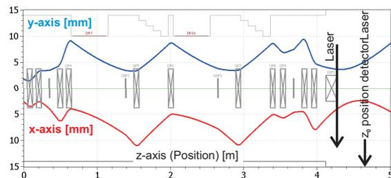
Figure 4: Envelope with adjusted quadrupoles to transport beam through sector magnet and creating a waist in horizontal plane, end of the diagnostic magnet at  $\approx 4.8$  m.
