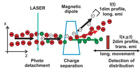
Figure 2: Basic principle of photo detachment ion beam diagnostics The  $H^-$  ions get neutralized by laser light. The diagnostics is in general a three stage process: detachment, charge separation and detector.
