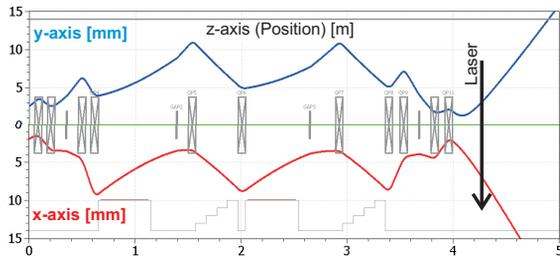
Figure 3: Envelope in x and y direction. The MEBT matches the beam to a future DTL. The possible laser position is marked, at  $\approx 4.8$  m would be end of diagnostic section followed by beamdump(s).
