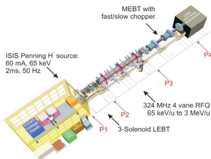
Figure 1: Overview of the FETS set up. The main elements are a Penning type ion source, 3 solenoid LEBT, RFQ and the MEFT consisting of quadrupoles, four buncher cavities and the chopper. The emittance diagnostic and beamdump are located at the end of the beamline.
