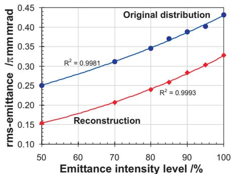
Figure 6: Comparison of the fractional emittance for several intensity levels. The difference is very likely ascribed to different numerical integrations (different number of particles).
