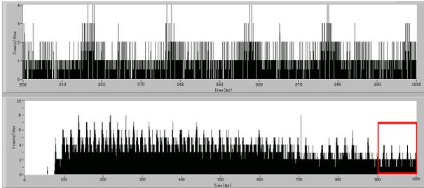
Figure 4: Spill structure (zoomed and total) measured by scintillator (sampling rate is 100 kHz, C6+, 200 MeV/u).
