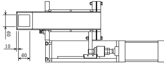
Figure 1: Detector pockets driven by pneumatics (CF150).
