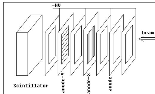
Figure 2: Structure of detector in pocket.
