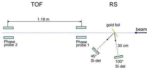
Figure 2.: Schematic presentation of beam energy measurement incorporated into the D-plate.
