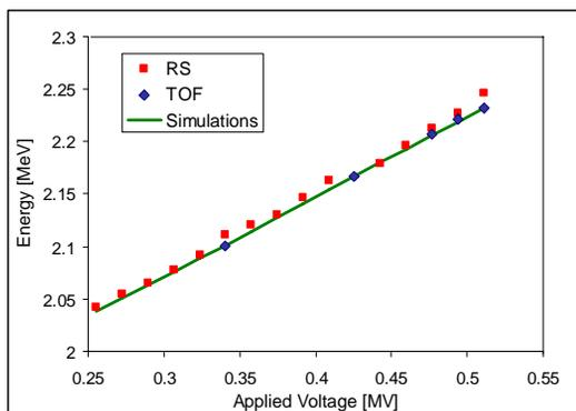
Figure 5: Proton energy as a function of HWR4 voltage, while the three previous resonators also operated.
