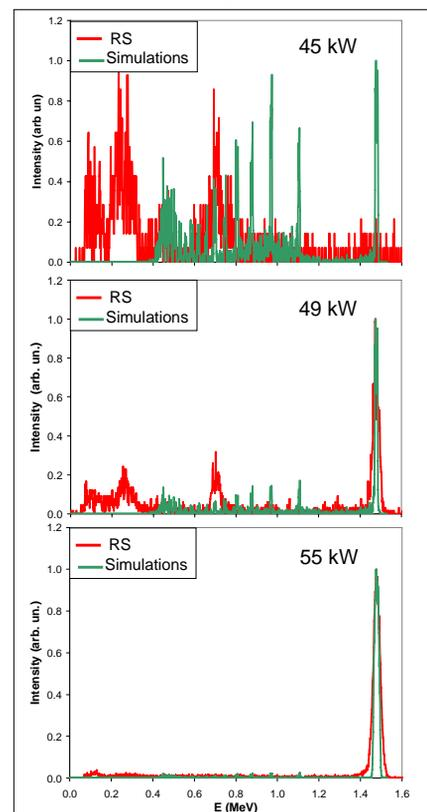
Figure 3: Evolution of proton energy spectrum for the turned off and detuned PSM resonators with increase of the RFQ RF power.
