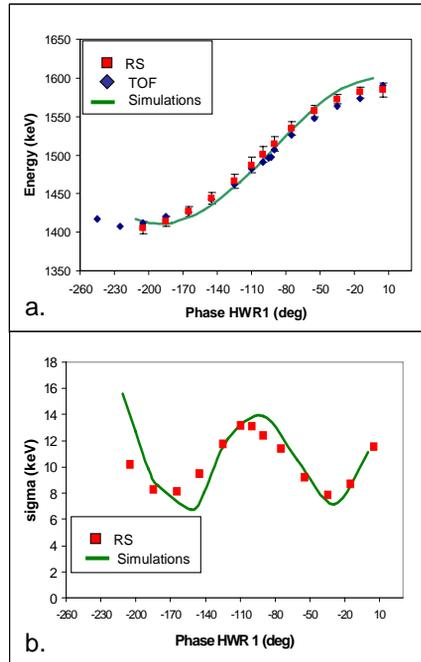
Figure 4: a: Proton energy as a function of HWR1 phase, as determined by TOF and RS b: Gaussian fit width (sigma) of the RS peak as a function of the HWR1 phase. Results are compared to the TRACK simulations.
