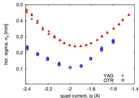
Figure 5: Hor beam sizes during a quad scan, inferred after analysis of the YAG and OTR images (MBM, 4 nC).
