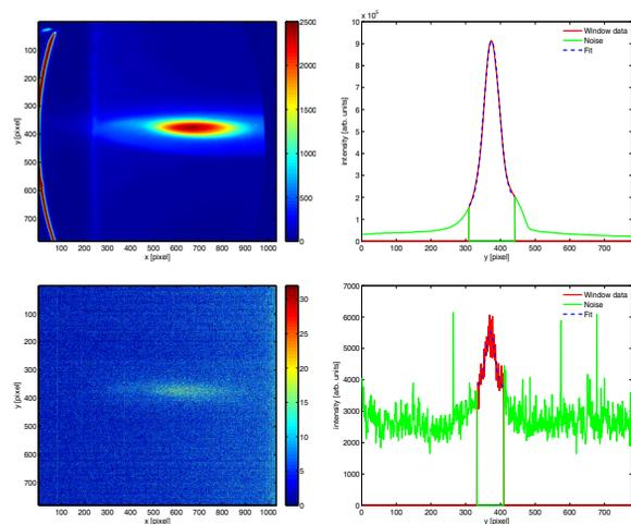
Figure 4: Two beam images and their profile analysis for the same Linac settings using the YAG (top) and OTR (bottom).
