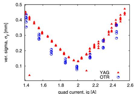
Figure 6: Ver beam size during a quad scan, inferred after analysis of the YAG and OTR images (MBM, 4 nC).
