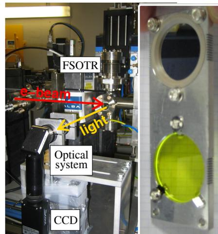
Figure 1: Picture of the FSOTR (right) installed at the Diagnostics line and screen holder with the YAG (bottom yellowish) and OTR screens (top).
