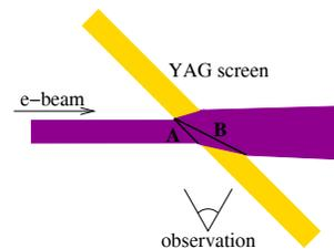
Figure 3: Beam size enlargement due to multiple scattering inside a YAG screen. The distance A appears as B.
