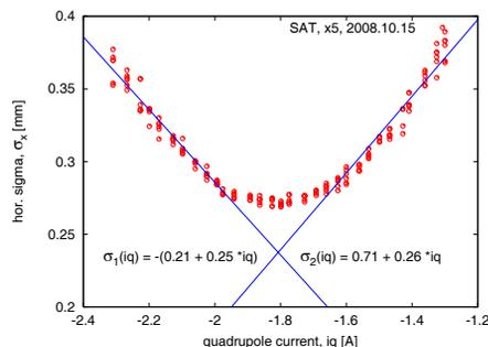
Figure 2: Beam size decreases linearly as we approach the beam waist (approximately at -1.8 A). Below 0.28 mm, the beam size enters a saturation regime. The blue line shows two linear fits to the data at each branch, and stresses the lack of linearity between -1.7 A and -1.9 A, which points the YAG saturation.
