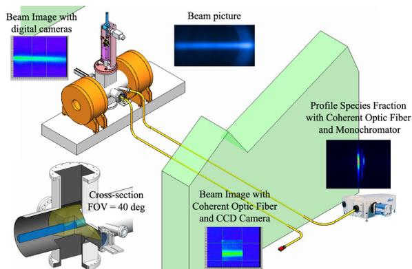
Figure 1: Methods of characterization of the deuteron beam of IFMIF Injector.
