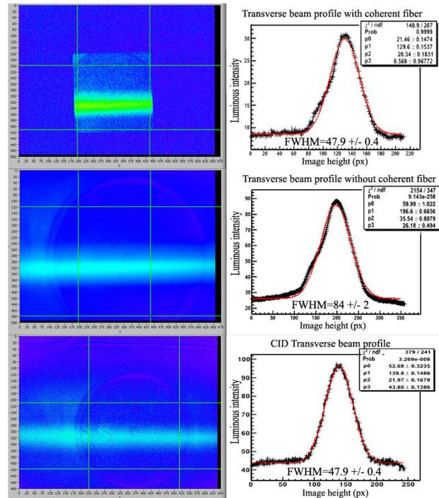
Figure 3: Obtained beam profile from image beam with coherent fiber and without and CID camera.
