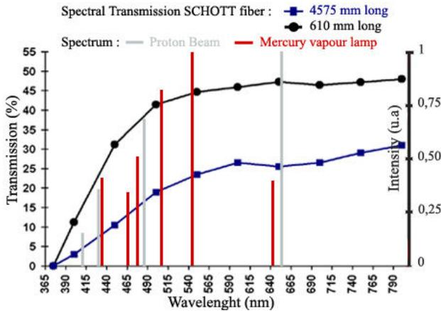
Figure 2: Spectral transmission for a SCHOTT coherent optical fiber of 610 mm and 4575 mm long, mercury vapor lamp and proton beam spectrums.
