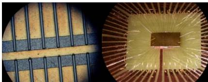
Figure 1: Magnified view of the IR array showing a few pixels of the photoconductive IR detector (left). Interface board and detector showing the connection between pixels and interface board made of gold bonding wires (right).
