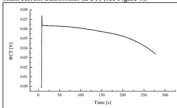
Figure 6: Beam current transformer signal.
