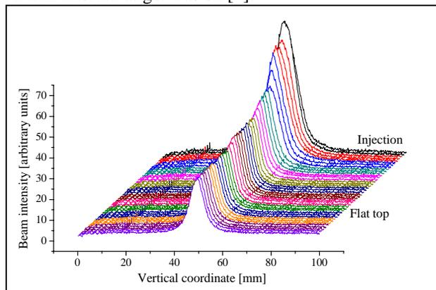
Figure 3: Evolution of the vertical proton beam profile during injection and acceleration to 1.343 GeV/c. About  $3 \cdot 10^9$  polarized protons reached flat top. Time span is 2 s.
