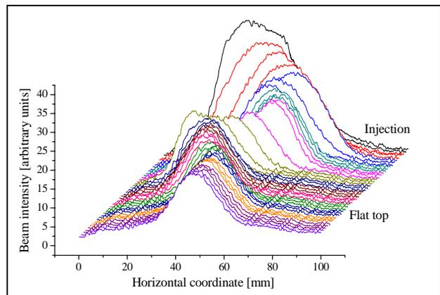
Figure 2: Evolution of the horizontal proton beam profile during injection and acceleration to 1.343 GeV/c. About  $3 \cdot 10^9$  polarized protons reached flat top. Time span is 2 s. Corrected for spatial detector sensitivity distribution via UV calibration. 5 pts moving average smoothing was applied.
