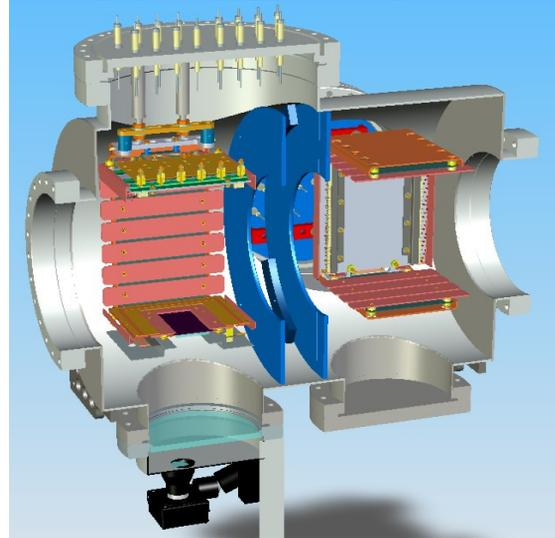
Figure 1: Mechanical design of the FAIR IPM prototype.
