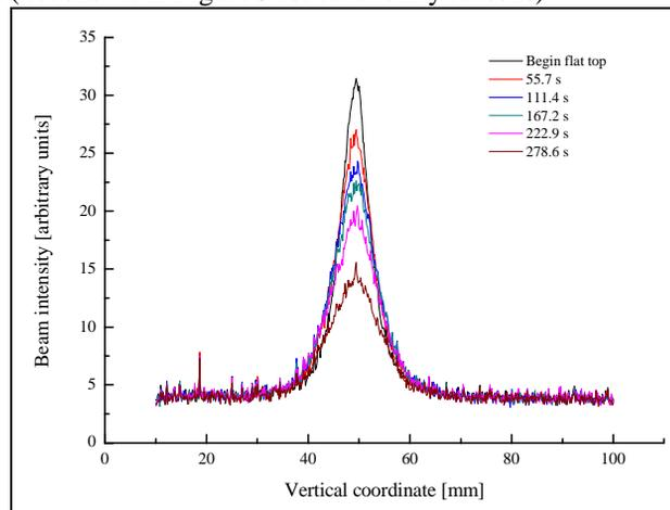
Figure 5: Vertical proton (polarized) beam profiles at 1.343 GeV/c flat top. Recorded during a 300 s COSY cycle with ANKE internal target on.
