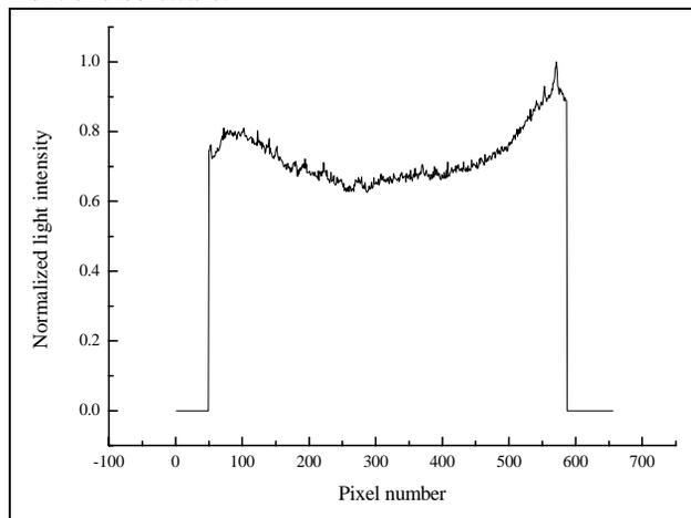
Figure 9: An example of the detector sensitivity distribution measured by illuminating the MCP surface with UV light and observing the PS light with the camera.
