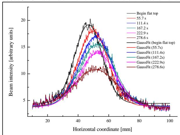
Figure 4: Horizontal profiles of the polarized proton beam at 1.343 GeV/c. The profile measurement started once the flat top was reached. COSY was operating in a 300 s cycle for ANKE experiment. Internal target on.
