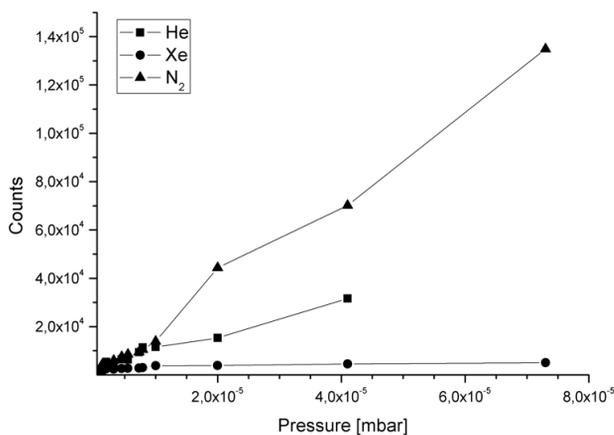
Figure 4: Photon yield for different gas pressures for He (●),  $N_2$  (▲) and Xe (■) at 12keV He ion beam.
