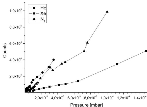
Figure 5: Photon yield for different gas pressures for He (●),  $N_2$  (▲) and Xe (■) at 6keV He ion beam.
