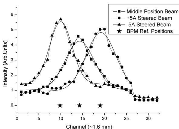
Figure 6: Profile measurements for a 3.14 MeV proton beam shifted with a steerer. The BPMs middle position is adjusted to fit the PMTs one. The channels on the right side are darkened for background measurement.
