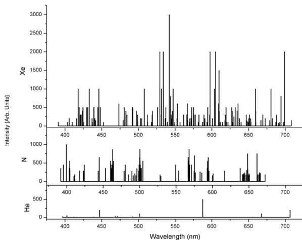
Figure 3: Expected wavelength distribution within the visible range of the investigated gases [3].
