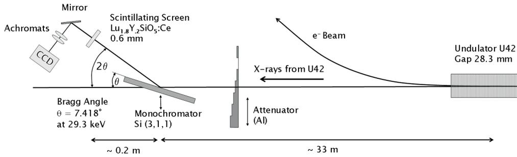
Figure 1: Sketch of the experimental setup seen from the top.
