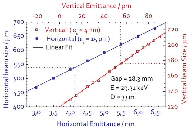
Figure 3: Horizontal and vertical rms beam sizes calculated with SRW for different emittance values.
