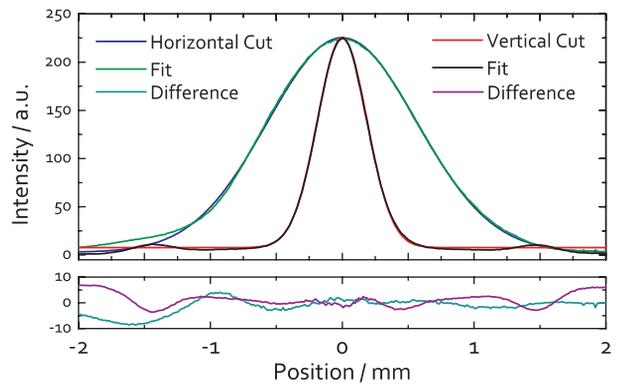
Figure 2: Horizontal and vertical cut through the measured beam profile, the lineouts of the fitted 2-dimensional Gaussian, and their differences.
