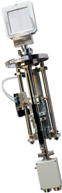
These monitors are composed of an horizontal and a vertical grid of golden tungsten wires of 150 μm.
