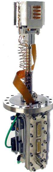
The principle of this profiler is based on the ionization of the residual gas of the lines by the beam. This diagnostic gives a one-dimensional profile and is composed by a drift space and a signal amplification stage (one micro-channel plate) with an anode of 35 strips spaced by 0.3, 0.5 or 1 mm. The working pressure is 10<sup>-8</sup> mbar and the desired resolution is 1mm. In order to obtain a low out-gassing, the profiler should be baking at 150 °C.
