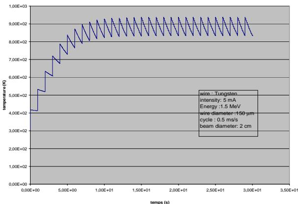
Figure 4: Temperature variation vs beam time on wire.
