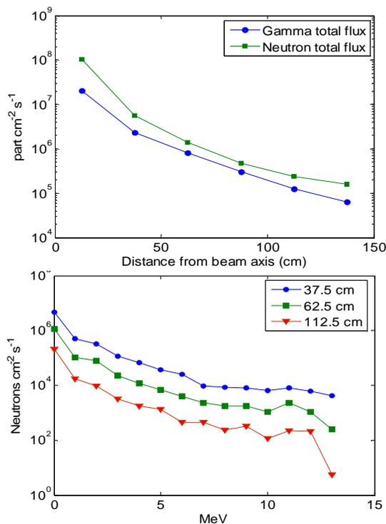
Figure 2: Preliminary estimation of total gamma and neutron fluxes versus the distance from the beam axis (top) and neutron spectra at 3 different distances from the beam axis (bottom) near the beam dump [9].
