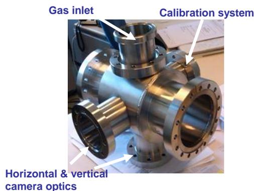
Figure 1: Illustration of the prototype vacuum chamber for the fluorescence profile monitor, showing the vertical and horizontal viewports, as well as those for gas injection and calibration.
