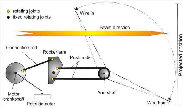
Figure 4: Schematic of a wire movement.
