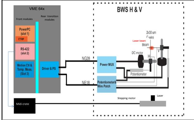
Figure 3: Electronics schematics of the calibration bench.
