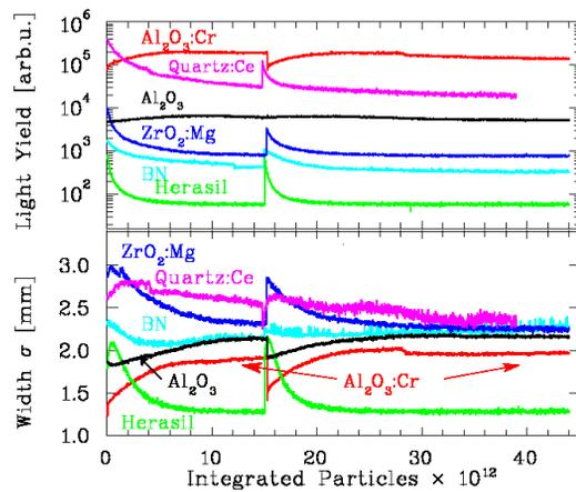
Figure 1: Light yield and beam width for different materials irradiated by 2200 macro-pulses of  $Ar^{10+}$  ions with  $2 \cdot 10^{10}$  ppp, in  $100 \mu s$  pulse length with 2.6 Hz repetition rate at 11.4 MeV/u ( $\sim 300 \mu A$ ). After 5 min. of irradiation, a 3 min. break was introduced to let the screen cool down, followed by 10 min. irradiation.
