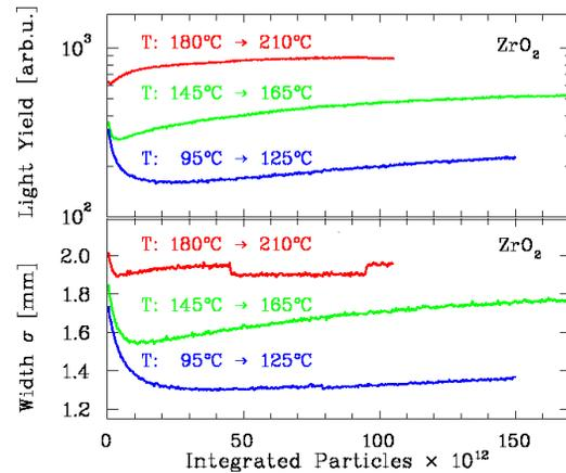
Figure 2: Light yield and beam width for  $ZrO_2$  irradiated by 300-500 macro-pulses of 2 Hz repetition rate with  $3.9 \cdot 10^{11}$  ppp  $H^+$  in 4 ms pulse length at 4.8 MeV/u.
