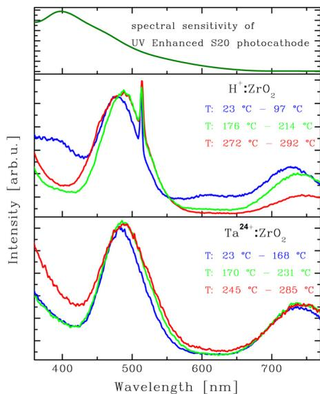
Figure 4: Spectra of  $ZrO_2$  for irradiation with  $Ta^{24+}$  and  $H^+$  ions for different heating levels. The beam parameters and the evaluation are the same as in Fig.3.
