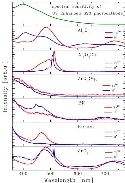
Figure 3: Spectra of the scintillators for  $Ta^{24+}$  (in red) and  $H^+$  ions (in blue). Beam parameters for  $H^+$ :  $4.1 \cdot 10^{11}$  ppp at 4.8 MeV/u, 2 ms pulse length, 2 Hz repetition rate. Beam parameters for  $Ta^{24+}$ :  $8.8 \cdot 10^9$  ppp at 11.4 MeV/u, 100  $\mu$ s pulse length, 1 Hz repetition rate. The spectra are averaged over about 1000 images and they are not corrected by photocathode (top) and spectrometer efficiency.
