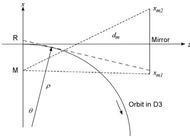
Figure 1: Radiation from a point inside the dipole. The plot also shows the acceptance of a slit placed
