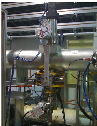
Figure 4: Electron scanner installation.
