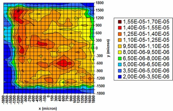
Figure 7: Quantum efficiency map of the SPARC photocathode obtained by data automatically collected through photo-injector control system.
