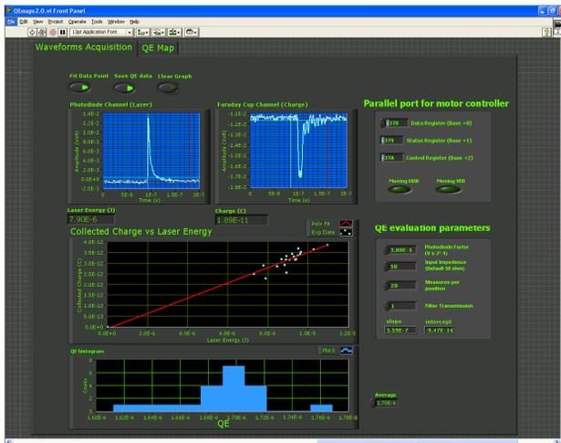
Figure 6: Picture of the front end software at console level used to acquire the emission curves of the photocathode.
