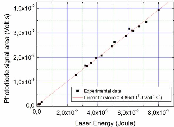
Figure 1: Typical calibration curve for the laser photodiode.
