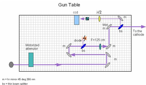
Figure 2: Layout of the final part of the laser beam transfer line. The position of the beam splitter and photodiode is also shown.
