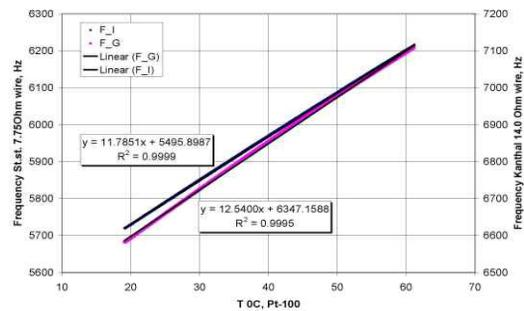
Figure 2: Calibration of two-wire VWM: magenta – Kanthal, blue –stainless steel.
