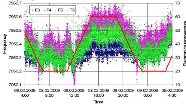
Figure 6: Comparison of the different electronic units with the same VWM sensor.
