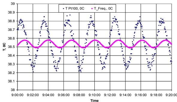
Figure 3: Thermostat on mercury thermometer base: signals from Pt100 and VWM are presented.
