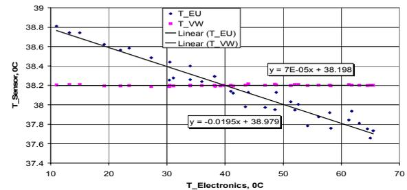
Figure 5: Comparison of the Pt100 and VWM readings dependences on electronics temperature.
