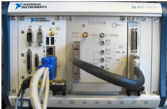
Figure 7: PXI Chassis containing an Embedded System Controller, the BunchView module and the FPGA card.
