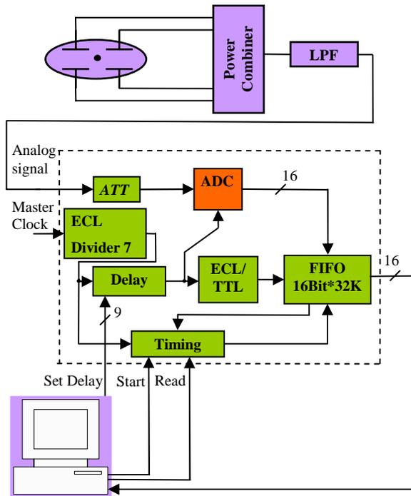
Figure 6: Hardware of the measurement system BunchView.
