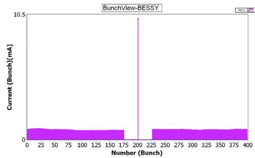
Figure 8: Typical Hybrid fill-pattern at BESSY measured with the BunchView system.
