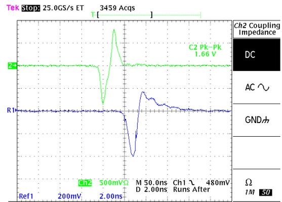
Figure 4: Voltage signals from stripline (in green) and ring electrode (in blue) for a single bunch (0.4 mA) circulating in the storage ring BESSY acquired by a real-time oscilloscope with bandwidth of 500 MHz.
