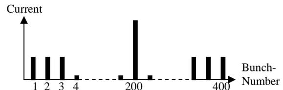
Figure 1: Fill-pattern in the storage ring.
