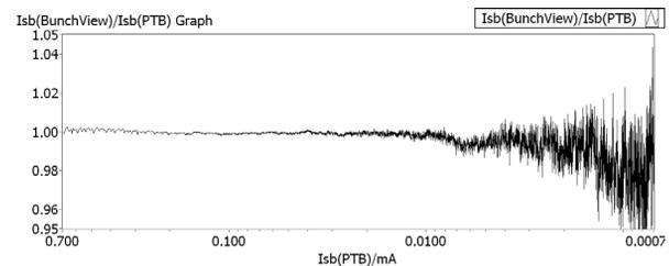
Figures 9: Confirmation of the very good linearity and high sensitivity of the BunchView system between 0.7 mA and 700 nA.
