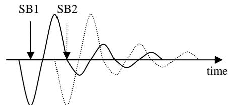
Figure 5: Sampling of the signal from equally populated neighbouring bunches. Signal interference has been reduced with a LPF.
