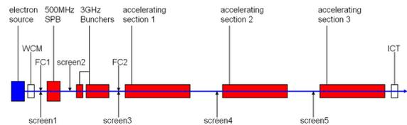
Figure 1: Functional block diagram of the linac diagnostic devices.
