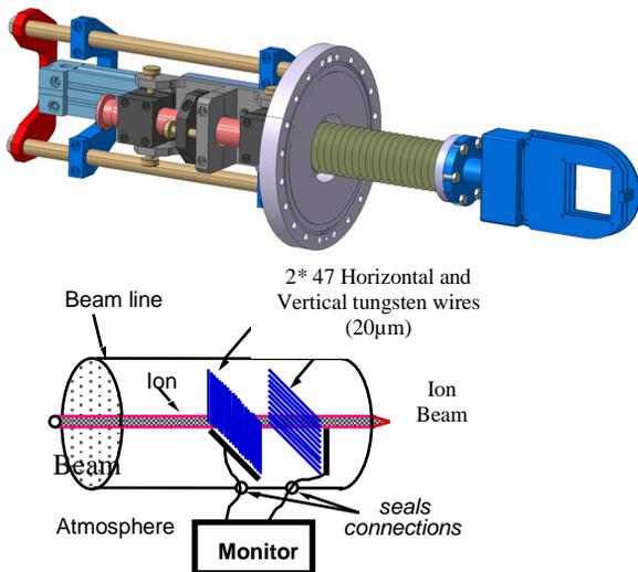
Figure 4: Secondary emission multiwire monitor, principle and picture.
