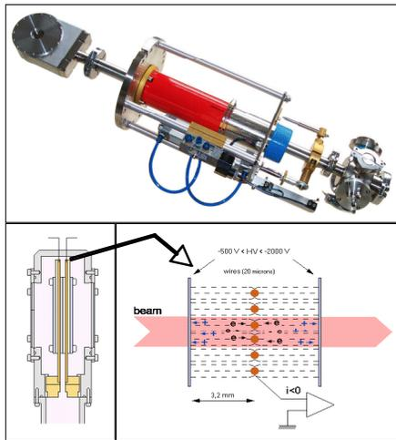
Figure 9: Gas Profiler: view and principle.
