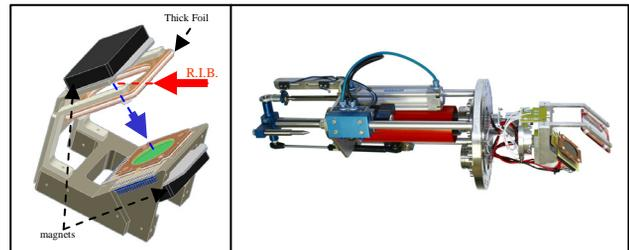
Figure 8: Secondary emission foil profiler: principle and view.
