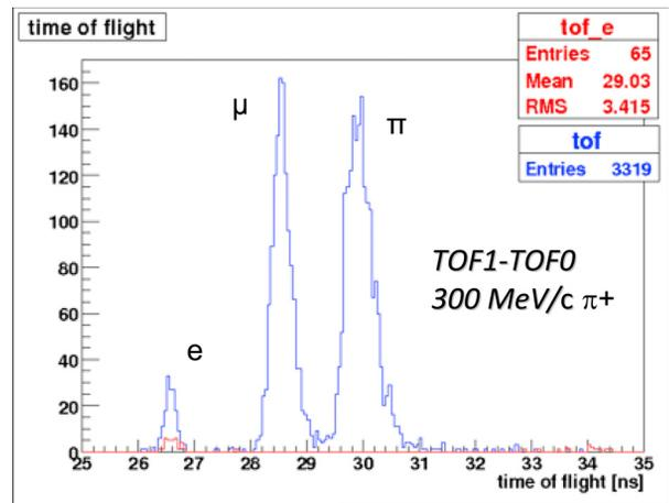
Figure 6: Time of Flight between the TOF counters for a positron (red) and pion (blue) beam.
