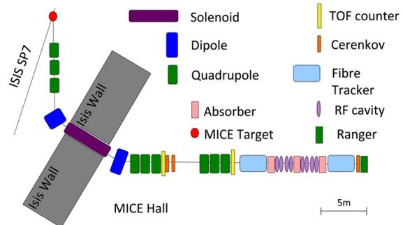
Figure 1: Schematic of MICE beam and cooling channel.
