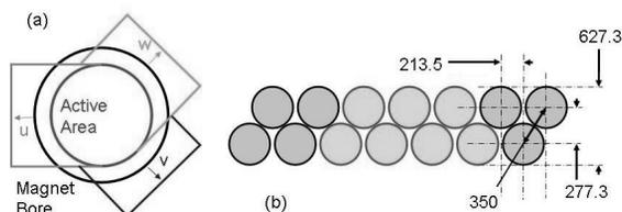
Figure 2: a) Three views per station. (b) Doublet layer shaded fibres bundled to form one channel (all distances in microns).
