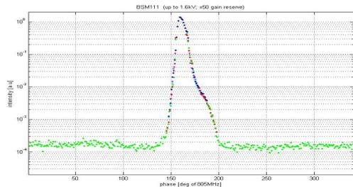
Figure 4: Longitudinal bunch profile measured in CCL.
