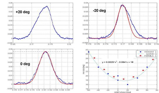
Figure 6: Bunch profile measurements in the SNS MEBT. Plots on top are for the buncher phase shifted from the nominal set point. Bottom left is for the nominal buncher setting. Bottom right is comparison of RMS bunch width vs. buncher phase dependence with the PARMILA simulation.
