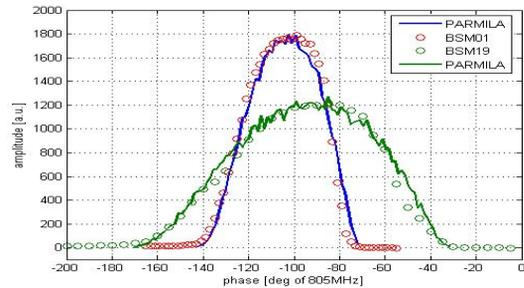
Figure 5: Longitudinal beam profiles measured in the HEBT compared to simulation.
