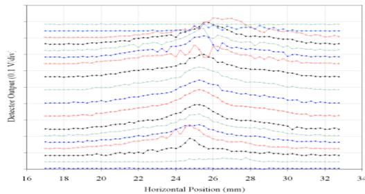
Figure 3: Transverse beam profile in the SCL measured with 20 nsec steps within a single mini-pulse.
