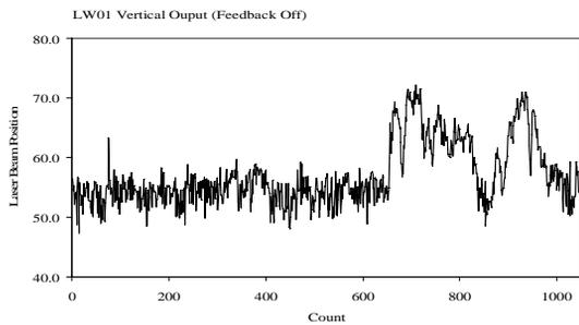
Figure 2: Laser beam position (arbitrary units) vs. time (1 sec/count) in the SNS Laser Wire system.
