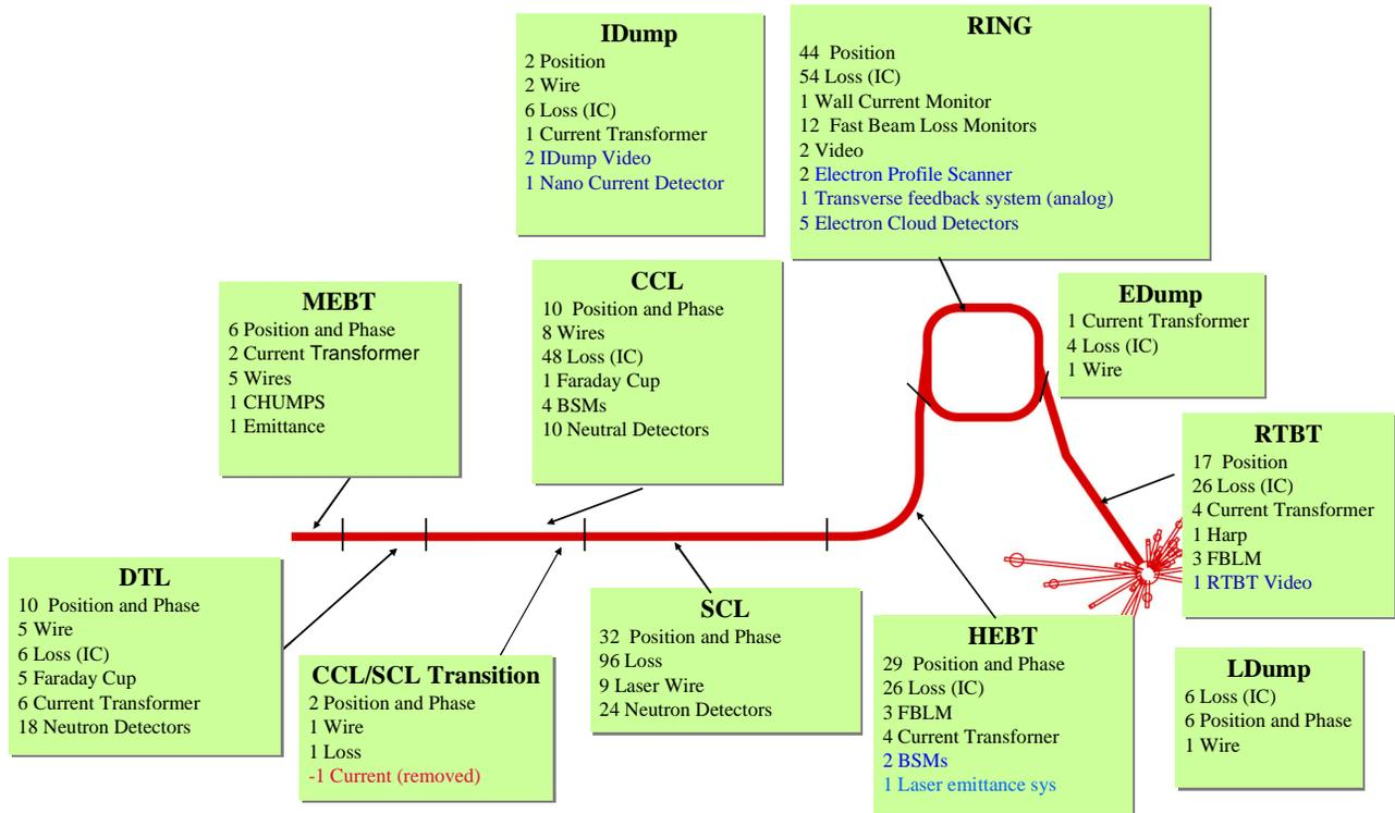
Figure 1: SNS Beam Diagnostics.
