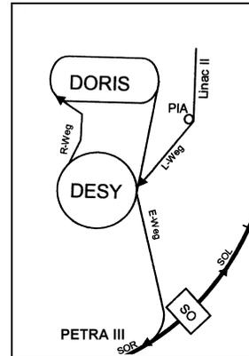
Figure 1: Petra III preaccelerator chain at DESY (Linac II, PIA, L-Weg, DESY II, E-Weg).
