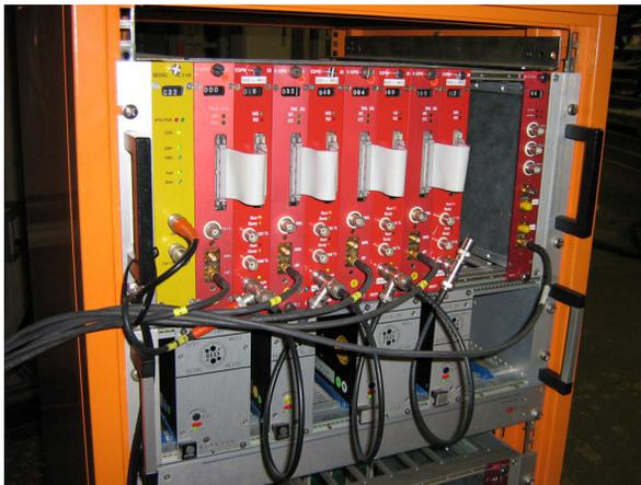
Figure 5: typical modular BPM system crate example (4 BPM channels).
