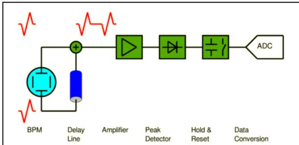
Figure 3: delay-multiplex single path technology (DMSPT) BPM signal acquisition principle [3].
