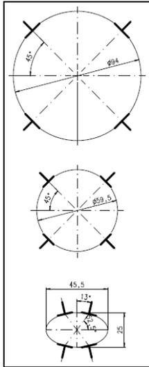
Figure 2: Vacuum chamber cross sections for the new BPMs.
