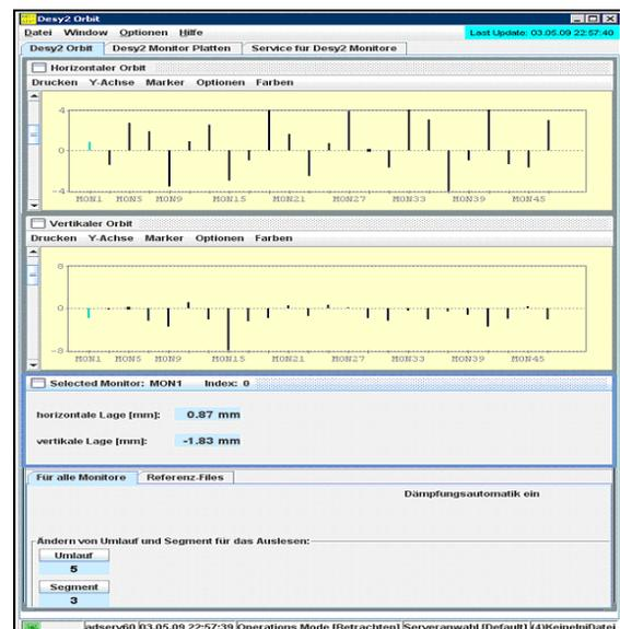
Figure 6: BPM application program example (client).
