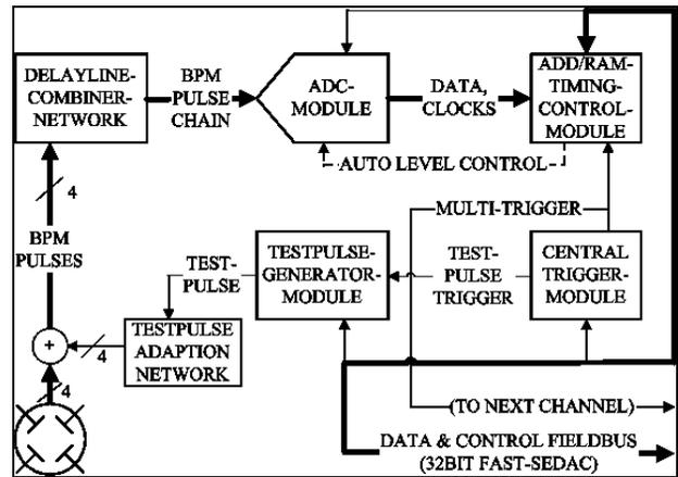
Figure 4: modular BPM single channel system setup.
