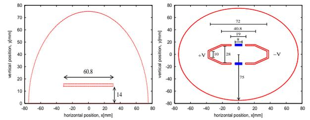
Figure 5: Transverse geometry of the vertical (right, half-geometry) and horizontal kickers (right).
