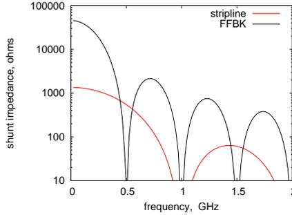
Figure 3: Shunt impedance of the stripline and vertical feedback kicker.
