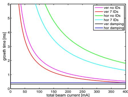
Figure 6: Damping rate needed for both planes for different machine configurations at zero chromaticity.
