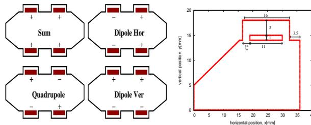
Figure 2: Independent modes in a four-electrode stripline (left), and geometry of one fourth of it (right).
