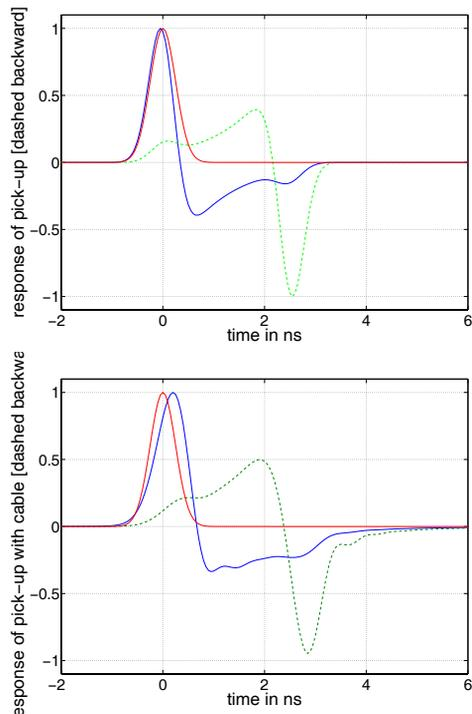
Figure 2: Pick-up response to gaussian bunch without and with cable. Red line represents the bunch intensity, blue and dashed line the signal distortion of a forward and backward pickup installation respectively.
