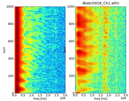
Figure 5: Evolution of spectra (sum and difference) for one LHC bunch in a bunch train subject to e-cloud transverse instability.
