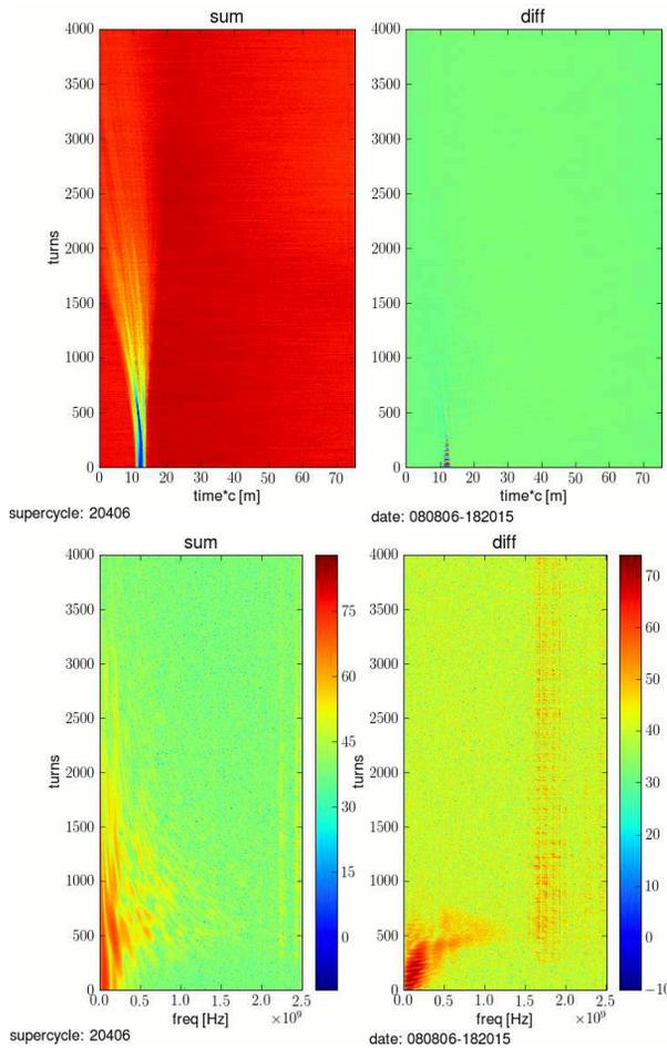
Figure 3: Debunching in the SPS, time domain data reconstructed and spectrum of sum and difference signal from a vertical pick-up. Bunch is unstable and lost.
