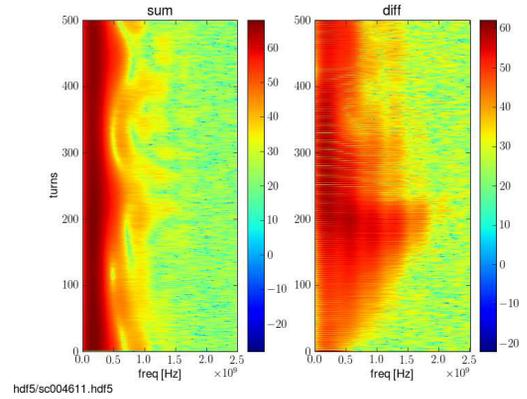
Figure 4: Evolution of spectra (sum and difference) for captured single bunch, transversely unstable.
