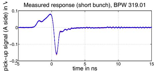
Figure 1: Measured pick-up response to single short bunch (backward installation).
