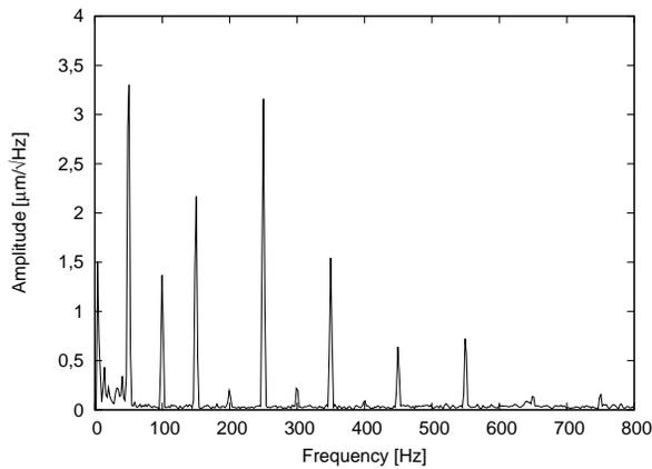
Figure 2: Spectral rms orbit deviation versus frequency.
