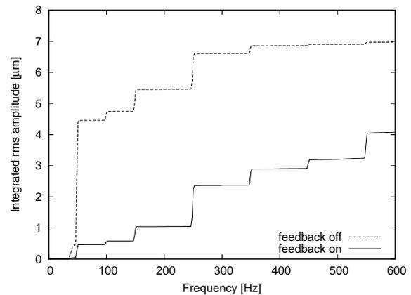
Figure 6: Integrated rms ampl. with feedback on and off.
