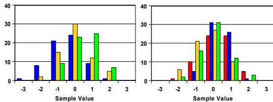
Figure 2: Histograms of AD6645 readings. Left/right, without/with awakening pulse.
