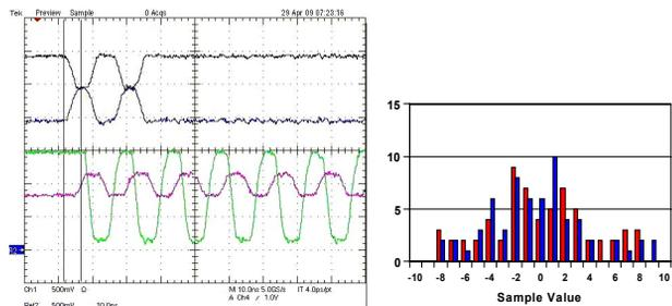
Figure 4: Left, the signals at the ADC inputs (top), the CLK signal (pink), and the DRY signal (green). Right, the pulse magnitudes (means are subtracted).
