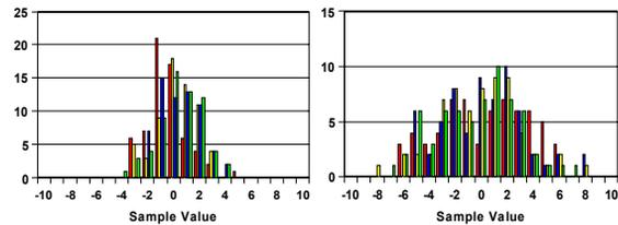
Figure 3: ADC readings noise with differential amplifier (left) and of full circuit (right).
