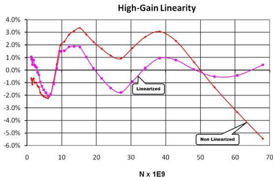
Figure 6: Linearization graph from the test bench.
