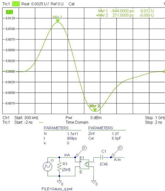
Figure 3: Measured pulse response of the LHC button pick-up and the electronic PSpice® simulation model.
