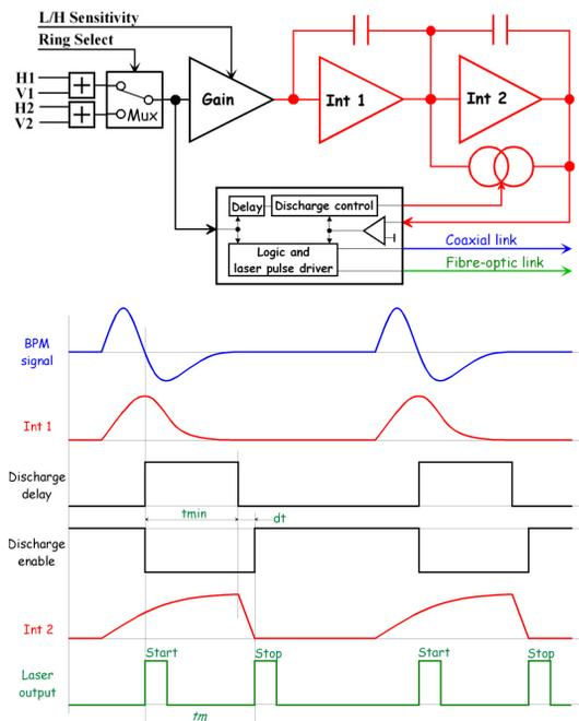
Figure 2: Intensity measurement principle and related waveforms.
