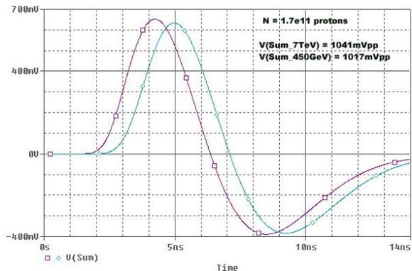
Figure 5: Simulated normaliser sum signal responses to the LHC bunch at 450 GeV and 7 TeV.
