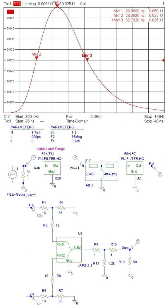
Figure 4: Network analyzer time-domain measurement of the normaliser sum-output and partial schematic of the equivalent simulation model.
