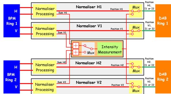
Figure 1: LHC position and intensity measurement system layout.
