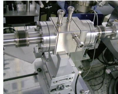
Figure 3: Photograph of the RF-BPM cavity.
