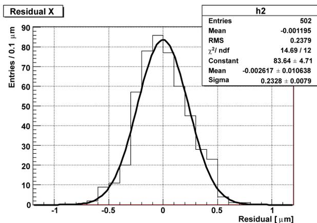
Figure 6: Residual distribution of the position resolution measurement. The histogram was fitted by a Gaussian.
