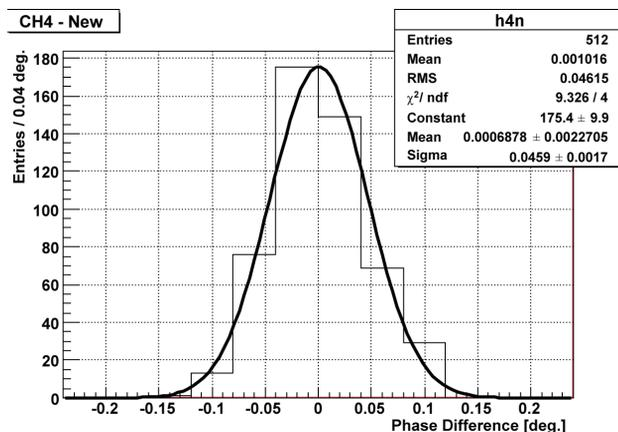
Figure 7: Phase difference between the TM010 cavities of the BPM 2 and 3. The histogram was fitted by a Gaussian.
