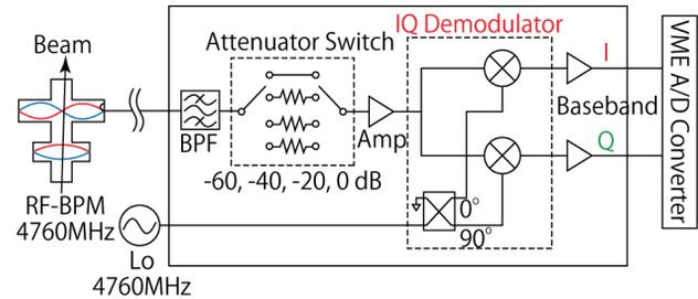
Figure 2: Block diagram of the RF-BPM electronics.
