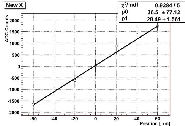
Figure 4: ADC count of the RF-BPM at each position. The error bars show the standard deviation of the histogram of the ADC data. A linear function fitted to the data is also plotted.
