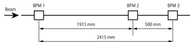
Figure 5: Arrangement of the three BPMs for the resolution measurement.
