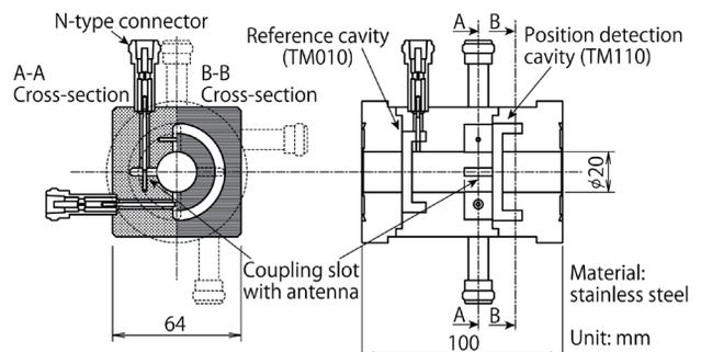
Figure 1: Drawing of the RF-BPM cavity.
