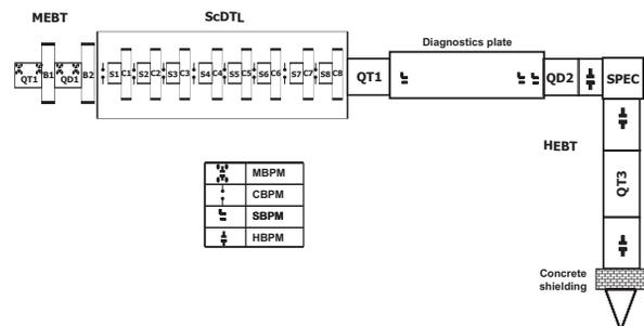
Figure 1: Distribution of the Beam Position Monitors along the accelerator.
