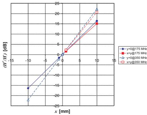
Figure 3: Simulation of the real part of the log-ratio method for the CBPM at  $\beta = 0.0728$  with  $\sigma_z = 15$  mm for the fundamental and first harmonic.
