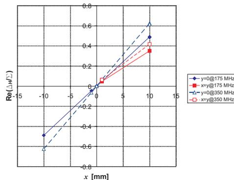
Figure 2: Simulation of the real part of the  $\Delta_H/\Sigma$  method for the CBPM at  $\beta = 0.0728$  with  $\sigma_z = 15$  mm for the fundamental and first harmonic.
