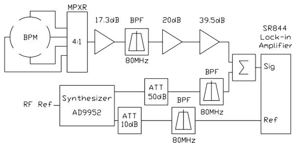
Figure 2: A simplified diagram of the signal processing equipment.
