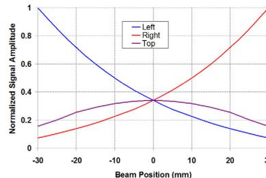
Figure 4: The calculated BPM signals as a function of horizontal displacement of a 10 mm diameter beam.
