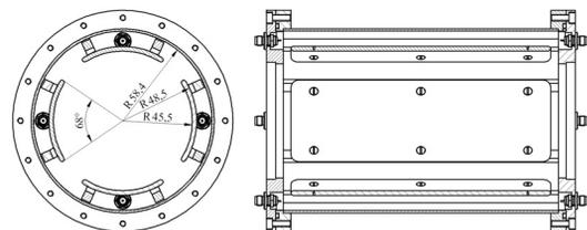
Figure 1: Cross-sectional views of the BPM.
