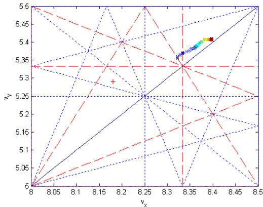
Figure 2: Booster tune drift during ramping.
