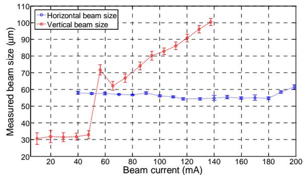
Figure 3: Beam size measured by interferometer.
