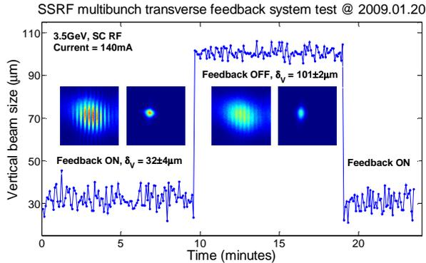
Figure 4: Measured beam size @ feedback on & off.
