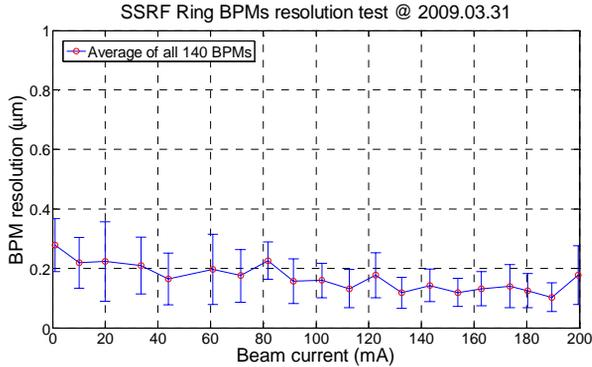
Figure 1: Ring BPM COD resolution test.
