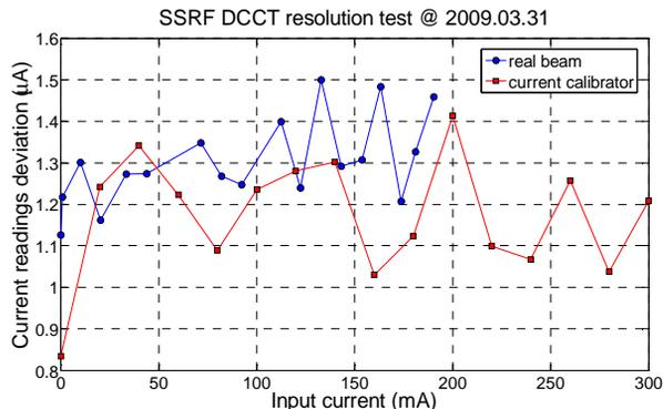
Figure 5: Ring DCCT resolution evaluation result.
