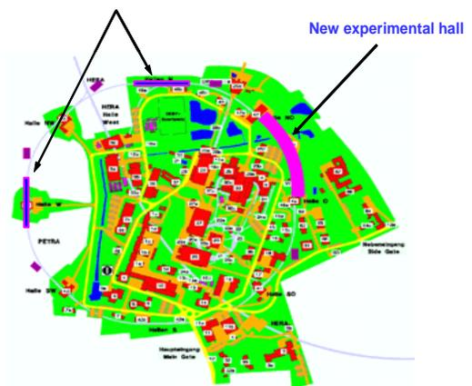
Figure 1: Ground Plan of the DESY site with the PETRA ring. The new experimental hall (purple) is situated between the PETRA halls North-East and East and the damping wiggler sections are in the North and West.
