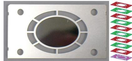
Figure 3: Thin stainless steel OTR screen.
