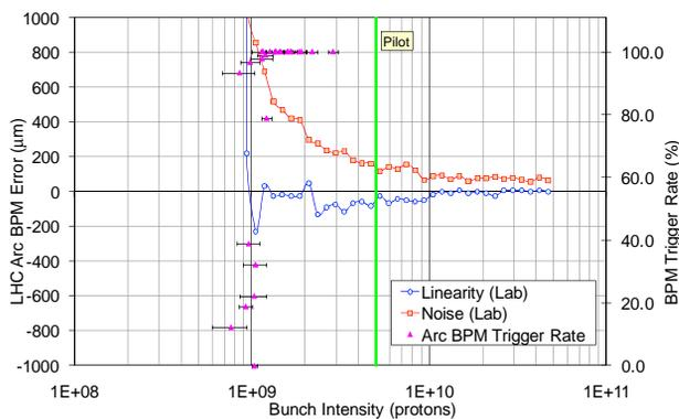
Figure 3 : BPM auto-trigger threshold determination – HIGH sensitivity mode (10/8/2008).
