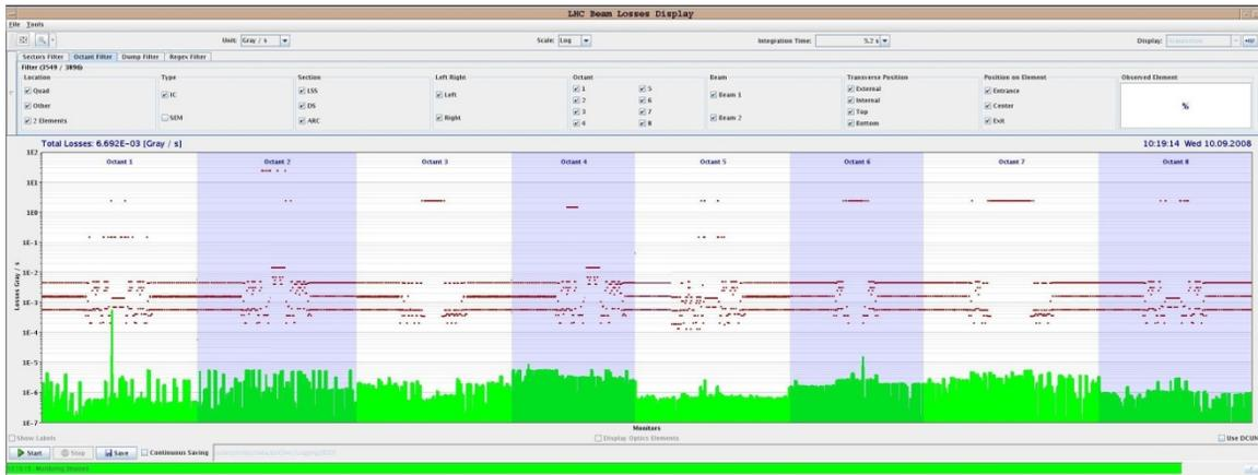
Figure 2 : BLM readings along the ring (logarithmic scale). In green the integrated signal from each ionisation chamber over the last 5.2 seconds updated every second. In red the corresponding threshold setting for each monitor.
