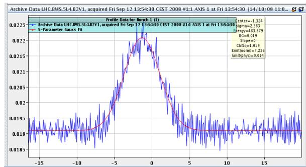
Figure 7 : Vertical wire scan on a single circulating pilot bunch (12/9/2008).
