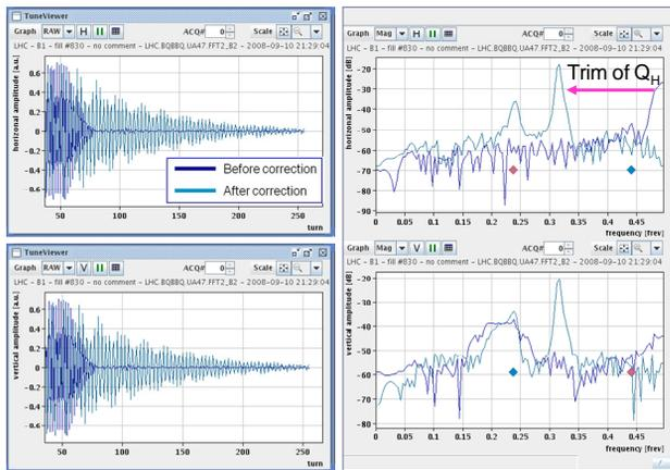
Figure 5 : First measurement and correction of tune using the LHC BBQ system.
