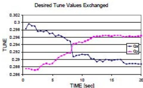
Figure 4: HERA tune controller: clear distinction of the working point even when crossing the tunes.
