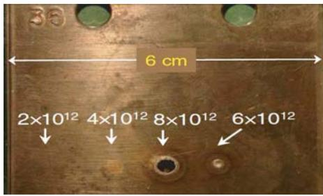
Figure 6: beam dump tests of a 450 GeV proton beam, being extracted from the SPS and dumped on a Cu target.
