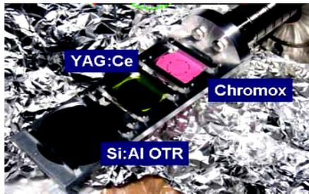
Figure 7: OTR and scintillating screens as diagnostic tools for low energy beams [7].
