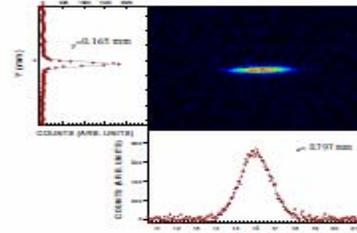
Figure 12: Synchrotron light image of the electron beam in the APS accumulator ring.
