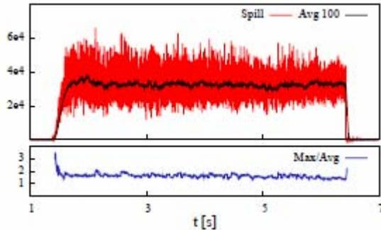
Figure 11: Measured particle flux during the slow extraction in HIT. The spill intensity corresponds to fractions of nA and has to be kept constant on a level of percent.
