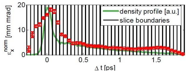
Figure 14: Slice emittance measurement at FLASH.
