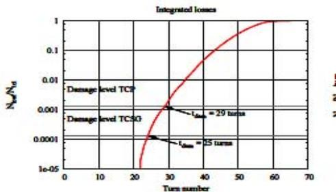
Figure 8: particle losses in LHC after a severe magnet failure: The damage level for machine components is reached already after 25 turns [8].
