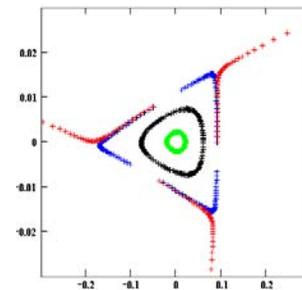
Figure 10: Schematic view in phase space of the slow extraction mechanism.
