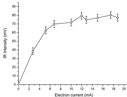
Figure 6: IR signal vs. the electron current.
