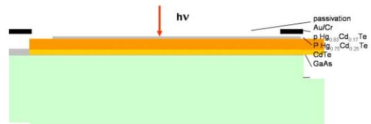
Figure 2 – Schematic cross section of an uncooled IR  $\text{Hg}_{1-x}\text{Cd}_x\text{Te}$  photodetector.
