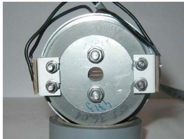
Fig. 5. VWM with tungsten wires and enlarged aperture.
