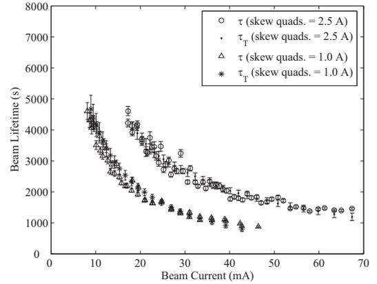
Figure 2: Touschek and total beam lifetimes for two skew quadrupole conditions. The dots/stars and circles/triangles correspond to the analyzed Touschek lifetime and the total beam lifetime, respectively, when the skew quadrupoles were set at 2.5/1.0 A.
