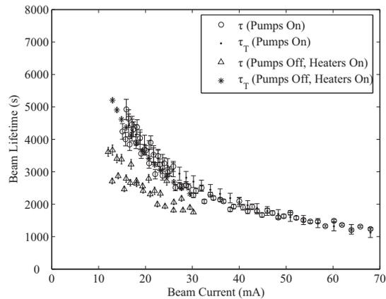
Figure 3: Touschek and total beam lifetimes for the same skew quadrupole condition (2.5 A) but different vacuum conditions. The dots and circles correspond to the Touschek lifetime and the total beam lifetime, respectively, under normal vacuum conditions (the same as for Fig. 2). The stars and triangles correspond to the Touschek and the total beam lifetimes, respectively, with all the SIPs and DIPs turned off and the baking heaters turned on.
