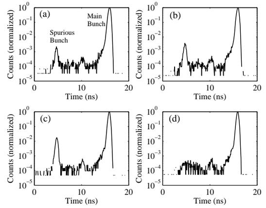
Figure 1: Change in temporal structure with time in single-bunch operation. Temporal structure (a) just after injection (total current 63.7mA), (b) after 10min(48.0mA), (c) after 87min (15.2mA), and (d) temporal structure without spurious bunches.
