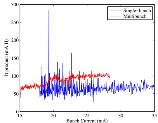
Figure 4:  $I\tau$  product in multibunch and single-bunch operation in the same condition. The multibunch operation has 12 bunches; the total beam current is 12 times larger than the bunch current.
