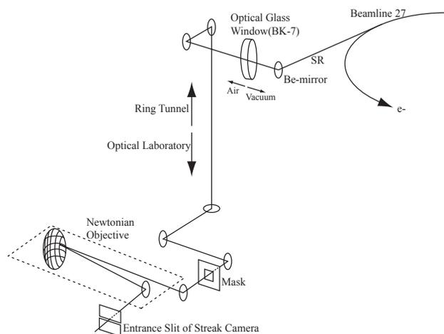
Figure 3: Optical layout of the bunch length measurement. The optical laboratory is located at the underground level of the storage ring.
