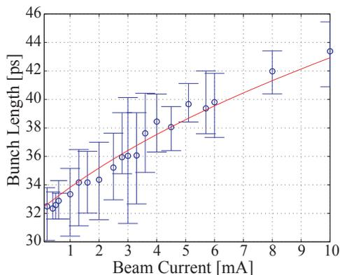
Figure 5: Bunch length at low beam currents. The solid line shows the fitted result with the potential-well distortion model.
