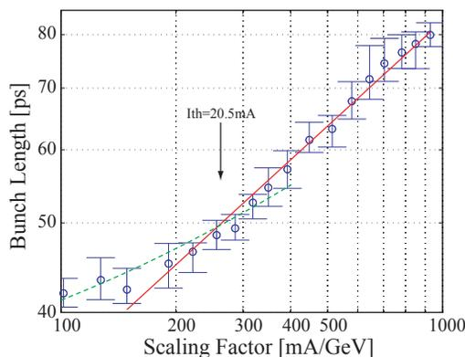
Figure 6: Bunch length above the threshold. The solid line and dotted lines denote the calculation using the scaling law and potential well distortion model, respectively.
