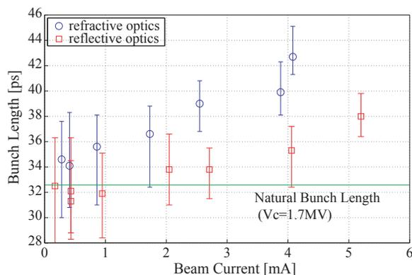
Figure 2: Bunch length difference with refractive optics and reflective optics. At low beam currents, the bunch length is close to its natural value obtained in the reflective optics measurement.
