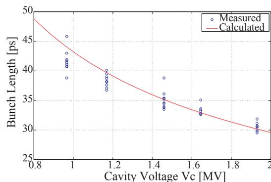
Figure 4: Bunch length as a function of cavity voltage at a beam current of 0.7mA. The solid line represents the calculated natural bunch length.
