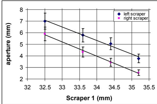
Figure 3: Dependence of the aperture measured by scraper 2 on the insertion depth of scraper 1.
