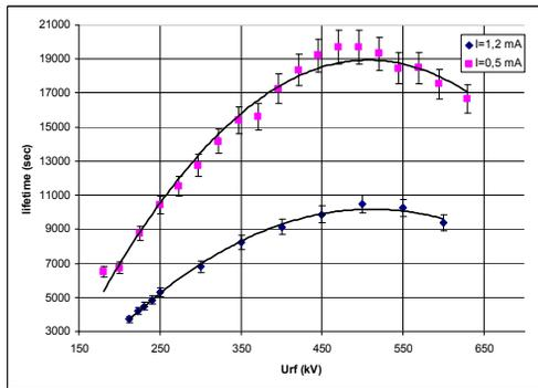
Figure 6: The dependence of the beam lifetime on accelerating voltage.
