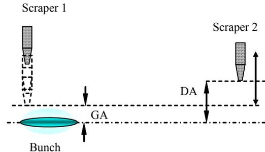
Figure 1: GA – geometrical aperture depended on the transverse coordinate of Scraper 1.
