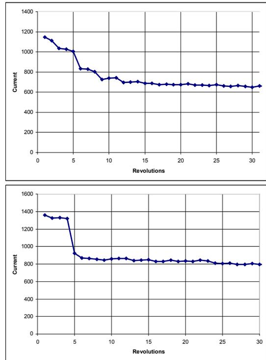
Figure 7: Beam loss at the dynamic (top) and mechanic (bottom) apertures.
