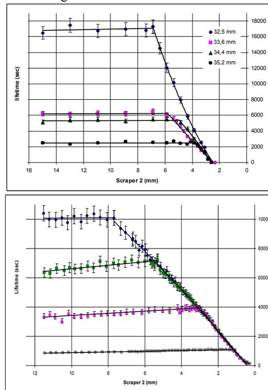
Figure 2: The beam lifetime dependence on horizontal (top) and vertical (bottom) positions of scraper 2 at different insertion depth of scraper 1.
