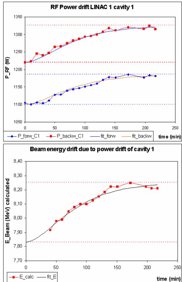
Figure 1a: RF power and mean beam energy drift after start up of the accelerator. ( $G_{C1} = 10$  MV/m,  $G_{C2} \approx 0$ ,  $E_{nom} = 8$  MeV)
