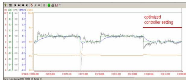
Figure 5: Optimizing the controller. (due value with added step function)
