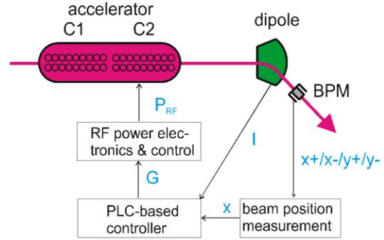
Figure 2: Scheme of the energy stabilization system. (C1, C2: Tesla cavities)
