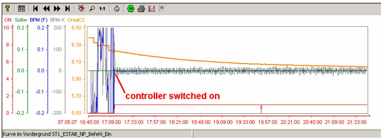
Figure 4: Operation of the energy control loop at  $E_{nom} = 14.5\text{MeV}$ ,  $G_{C1} = 10\text{ MV/m}$ ,  $I_{Beam} = 450\mu\text{A}$  in cw mode. (“ON”: controller on state, “Sollw”: BPM due value, “BPM(F)”: BPM reading filtered with 30 sec, “BPM-X”: BPM reading, “GRAD\_C2”: gradient set value for cavity 2 (controller output).
