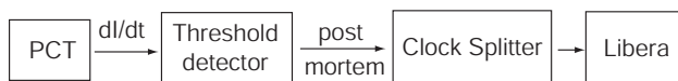
Figure 7: Setup for analyzing beam loss 'post mortem'. The beam loss trigger is generated from the differential output of a Parametric Current Transformer (PCT) used for beam current measurement.
