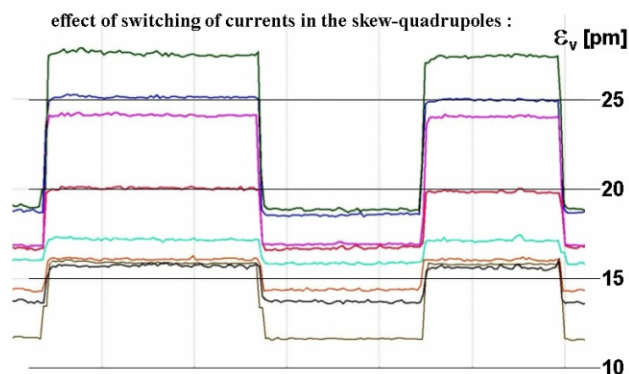
Figure 7: small result values of the 8 devices showing the effect of skew-quad current variation at high resolution.
