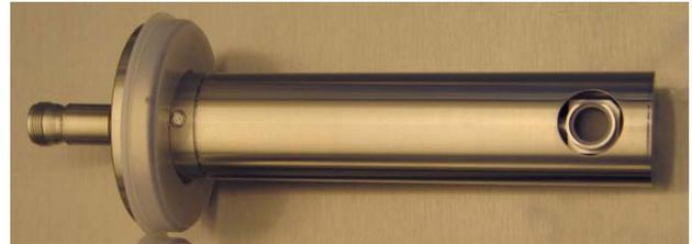
Figure 1: The linac faraday cup assembly
