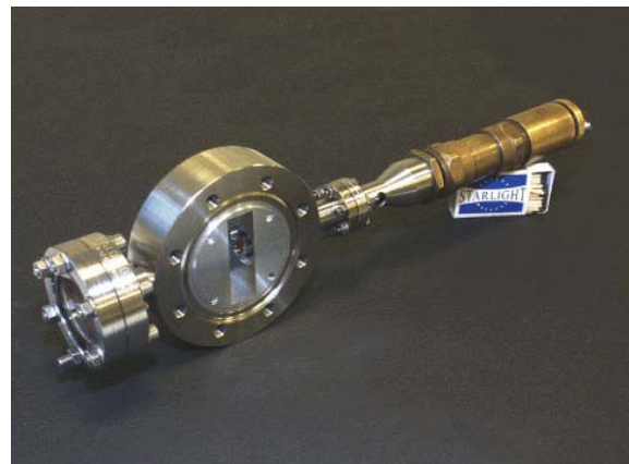
Figure 1: Photograph of the vacuum flange containing the EO sensor. The EO crystal together with two small metal mirrors are mounted on a translation stage (visible on the right). The entrance/exit window for the probe laser beam is visible on the left.
