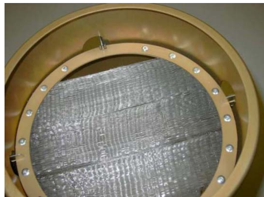
Figure 7: Sieve woven from diameter 0.1 mm and 0.3 mm tungsten wire.
