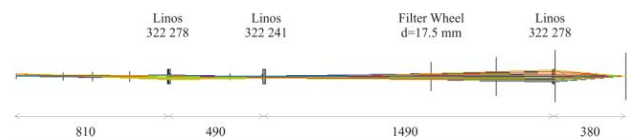
Figure 1: Overview of an optical line as it is presently used in CTF3
