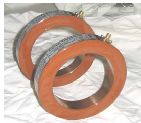
Figure 3: Picture of 2 Fast Current Transformers BERGOZ FCT-082-10:1-WB
