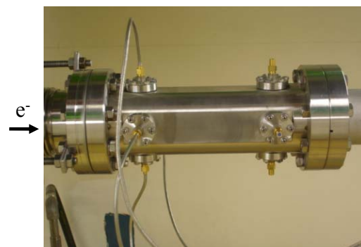
Figure 2: Stripline type beam position monitor
