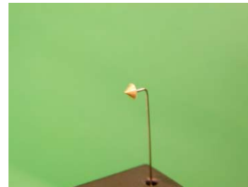
Figure 7: Photograph of the opaque disk to block the glare of central image.
