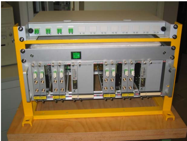
Figure 4: A BPMI front-end crate before installation in the tunnel. On the top can be seen the optical fibre patch panel.
