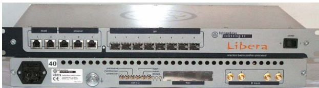
Figure 1: Front and back panels of a Libera chassis
