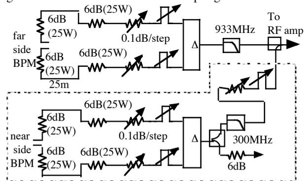
Figure 4: Front-end circuits for BPM with coupling canceller (inside of dotted line). The output of the circuits is send to an RF amplifier.
