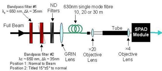
Figure 2: Optical arrangement employed to couple the synchrotron beam into the 4.3µm core fibre (single mode at a wavelength of 630nm) and optically image the photons onto the 50µm diameter SPAD.
