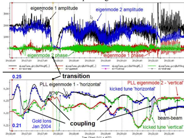
Figure 1: PLL tune tracking during a RHIC ramp.
