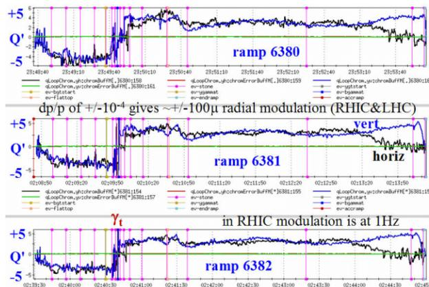
Figure 4: Chromaticity Measurement on the Ramp
