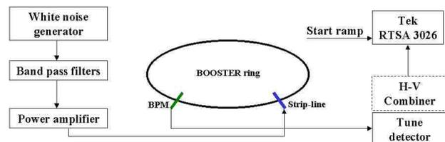
Figure 1: Fast Tune measurement system block Diagram
