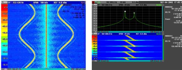
Figure 4 LEFT: spectrogram obtained in the laboratory showing a 250 KHz carrier, amplitude modulated ( $F_{mod}=25\text{ KHz}\pm 10\text{ KHz}$ ). RIGHT: laboratory spectrogram of a frequency swept carrier ( $f_c=982.8\text{ KHz}$ ) with a 160ms ramp ( $\Delta f=\pm 1.5\text{ KHz}$ ).
